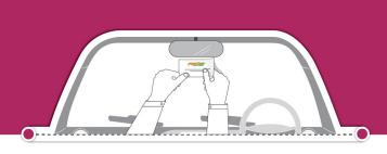
Install on the top middle centre of the windshield from INSIDE the vehicle (behind rear view mirror)
